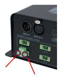
Begin by inserting the male end of the Phoenix connector into the desired signal output port on the driver, making sure that the latch on the Phoenix connector engages with the signal output port. Tighten the two screws located to each side of the wire terminals, as highlighted in the image to the above right.
