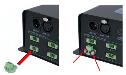
Begin by inserting the male end of the Phoenix connector into the desired signal output port on the driver, making sure that the latch on the Phoenix connector engages with the signal output port. Tighten the two screws located to each side of the wire terminals, as highlighted in the image to the above right.
