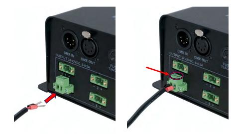
Now insert the wire leads from the fixture into the wire terminals of the Phoenix connector, making sure that the bare wire lead ends have been fitted with wire end sheaths. Tighten the two screws above the wire terminals, as shown in the image at above right, to secure the wire leads in the Phoenix connector.
