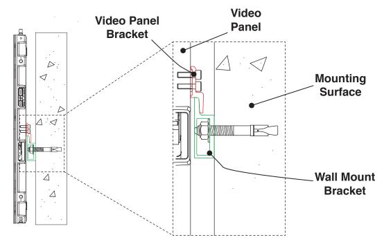
4. When mounting an assembly of multiple video panels, please note that wall mount brackets should be used for at least every other panel in a given vertical column. Brackets should extend across the full horizontal width of the panel assembly.
