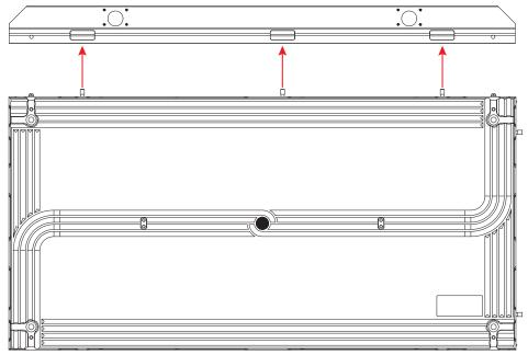
2. Place the panel on a secure, stable surface with the back facing up. Align one of the included plate brackets at the upper corner of the panel to connect the panel and the rigging bar. The upper hole of the plate bracket should line up with the hole on near the end of the rigging bar. Insert an M6x55 screw through the upper hole of the plate bracket and through the rigging bar, then secure in place with a matching nut on the other side of the rigging bar.
