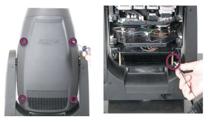
2. Use a Phillips head screwdriver to loosen the four (4) fasteners on each of the covers. Please note that these fasteners are of the twist-lock variety, and do not come free of the covers. Remove the safety cable clips securing each cover to the fixture.
