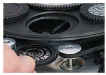
Rotate the Static GOBO Wheel until the desired GOBO is visible through the OPEN slot in the Rotating GOBO Wheel. Using a precision pick (or similar tool), carefully press the Static GOBO Holder down slightly, then using your thumb and index finger, gently pull it out and away until if fully clears the GOBO Wheel.
