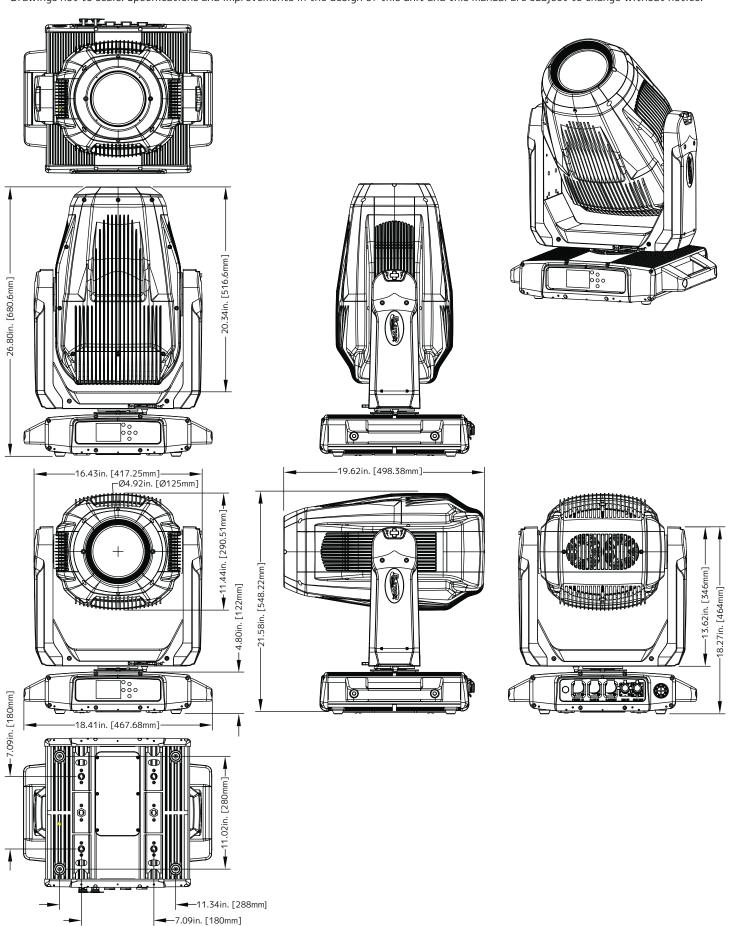
**DIMENSIONS**\*Drawings not to scale. Specifications and improvements in the design of this unit and this manual are subject to change without notice.
