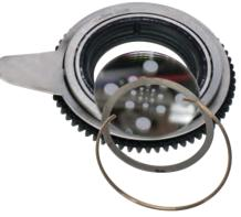
Locate the tab of the spring, and with a precision pick (or similar tool), carefully press the retaining spring inward to relieve the tension. Remove the retaining spring and carefully separate the GOBO from the GOBO Holder. Lastly, remove the flat washer attached to the removed GOBO and attach it to the desired replacement GOBO. Install the replacement Rotating GOBO following the steps above in reverse order.
