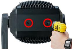
2. Remove (2x) Phillips-head screws on the bottom cover to expose the safety cables for the front and back covers. With bottom cover removed, remove the (10x per cover) Phillips-head screws on the front and back covers. One at a time, gently lift the covers and unclip the safety cables to remove them completely from the fixture.
