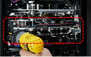
**3.** The GOBO Wheel module is secured to the fixture frame rail with (2x) sliding slotted brackets. To remove the module, loosen the (4x) Philips-head screws holding the brackets just enough (do not remove them) to allow the slotted brackets to slide down.
