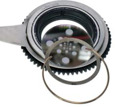
**8.** Locate the tab of the spring, and with a precision pick (or similar tool), carefully press the retaining spring inward to relieve the tension. Remove the retaining spring and carefully separate the GOBO from the GOBO Holder. Lastly, remove the flat washer attached to the removed GOBO and attach it to the desired replacement GOBO. Install the replacement Rotating GOBO following the steps above in reverse order.
