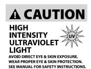
RISK GROUP 3 - RISK OF EXPOSURE TO ULTRAVIOLET UV RADIATION! FIXTURE EMITS HIGH INTENSITY WAVELENGTH OF ULTRAVIOLET UV LIGHT FROM THE UV LED. WEAR PROPER EYE AND SKIN PROTECTION. AVOID PROLONGED PERIODS OF EXPOSURE TO UV LED. AVOID WEARING WHITE COLOR CLOTHING AND/OR USING UV PAINTS ON SKIN.
