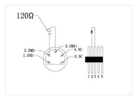
Termination reduces signal errors and avoids signal transmission problems and interference. it is always advisable to connect a DMX terminal, (Resistance 120 Ohm 1/4 W) between PIN 2 (DMX-) and PIN 3 (DMX +) of the last fixture.
