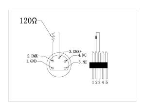
Termination reduces signal errors and avoids signal transmission problems and interference. it is always advisable to connect a DMX terminal, (Resistance 120 Ohm 1/4 W) between PIN 2 (DMX-) and PIN 3 (DMX +) of the last fixture.
