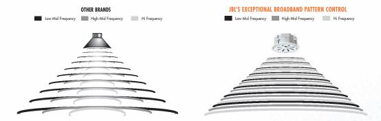
CONSISTENT COVERAGE Well-controlled wide coverage from the Control 47C/T and Control 47LP allows the use of fewer speakers, substantially reducing overall system cost, while providing more consistent sound throughout the listening space. Narrow, focused coverage from the Control 47HC allows use in high ceiling locations and highly reverberant spaces.
