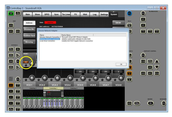
Choose either the LAN adaptor (for wired connection) or the Wireless adaptor, depending on how you are connecting the PC running Virtual Vi to the console. Then proceed to set up Mirroring as described in the preceding sections.
