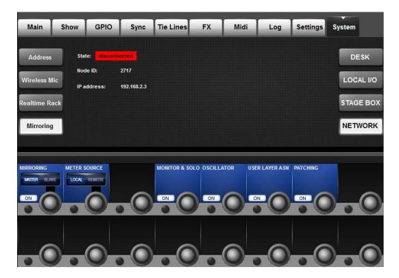
Before enabling Mirroring, decide which console will be the Primary and which the Secondary, and set the **PRIMARY/SECONDARY** controls accordingly on each console.
