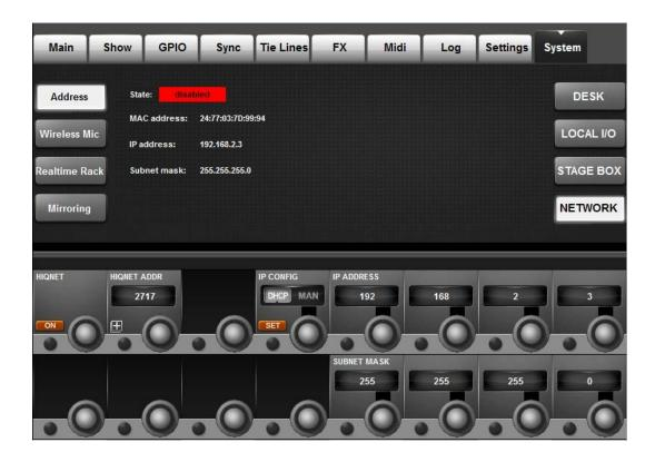
Select either MAN (manual) or DHCP (automatic) mode for setting the address, depending on requirements. Press the SET button after changing modes, or selecting the required address in manual mode, and wait for the address to be displayed in the upper section of the touchscreen.
