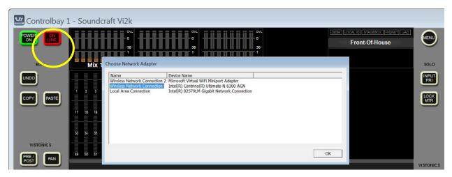
Note that no IP address setup is necessary when using the ONLINE button to connect to the Local Rack, because an appropriate IP address is automatically assigned to the network adaptor when the ONLINE mode is enabled. This is a temporary IP address and is removed when Virtual Vi is shut down. You do not need to change the IP configuration settings of the LAN port on the PC.
