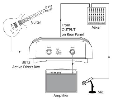
Example Setup 2: Direct guitar signal and amped signal on two mixer channels
