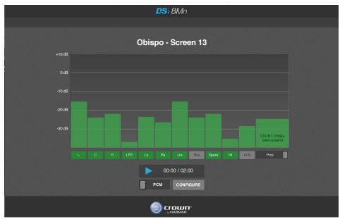
Figure 9 Remote Monitoring (Non-biamped)
